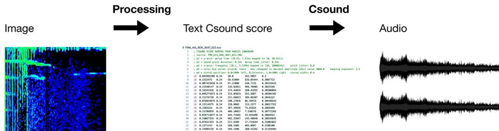
Figure 2: Pipeline for translating ionograms to a score of small sound grains using Processing, and compiling it with Csound to obtain a stereo audio file.
