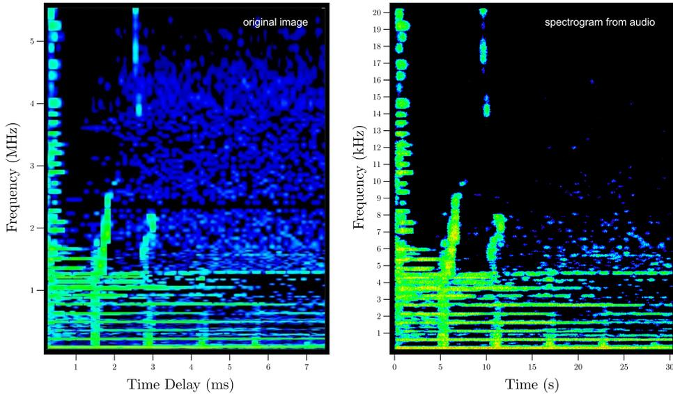
Figure 3: Comparison of an original ionogram with the spectrogram of its sonification. The graphs have been rotated 90 degrees to provide a more intuitive representation of the sound, with time on the horizontal axis.
