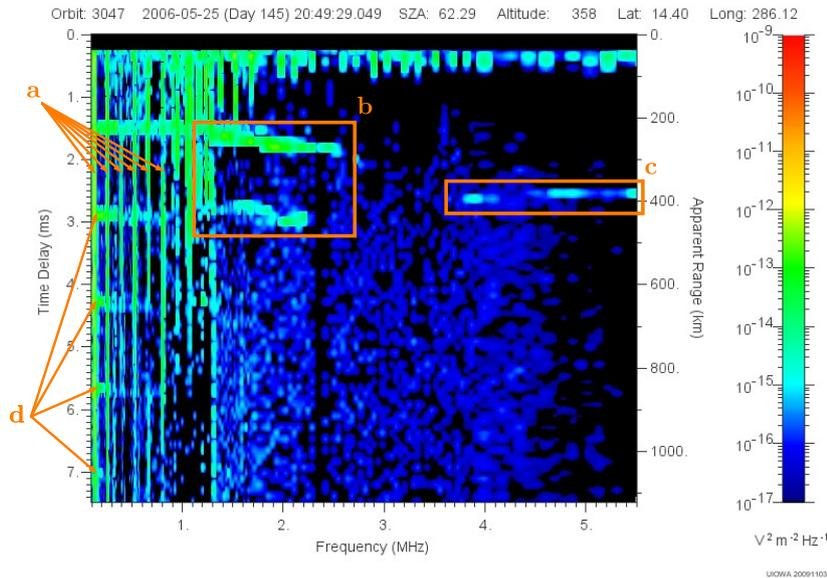
Figure 1: Main structures of the ionograms marked in orange: a) Harmonics produced by the interaction between MARSIS antennas and the ionosphere. b) Ionospheric traces around 1-3 MHz. c) Line at high frequencies due to reflection from Mars’ surface. d) Horizontal lines from electrons accelerated by the antennas’ electric field interacting with the ambient magnetic field (cyclotron echoes).
